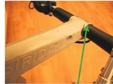
strida 2.5 – note exposed steel stem for folding handlebar compliance.
