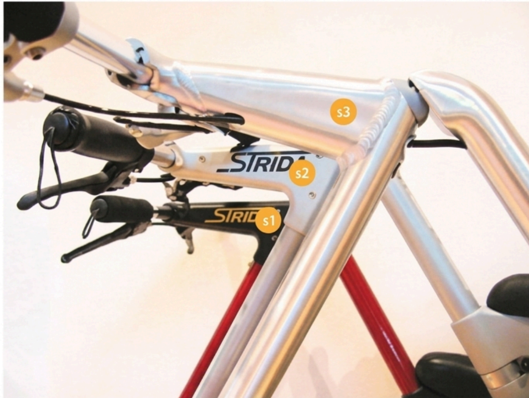
strida 2.5 – note exposed steel stem for folding handlebar compliance.
